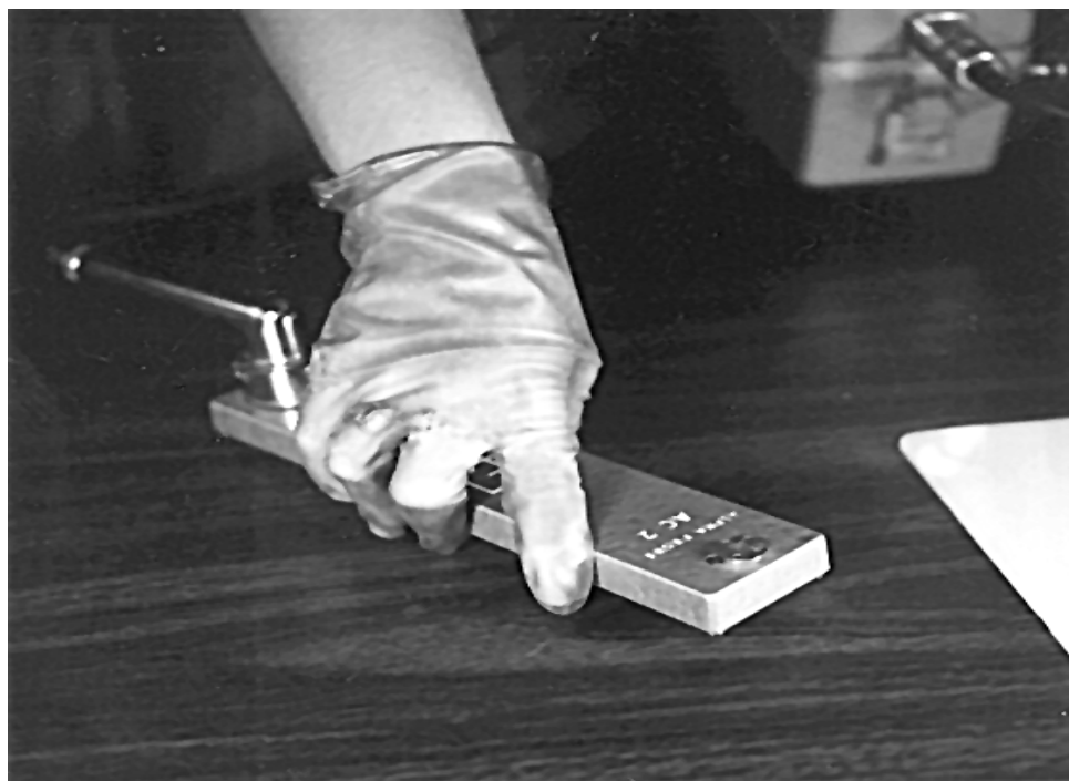
Fig. 8 - Technique to maintain a fixed distance from a surface
