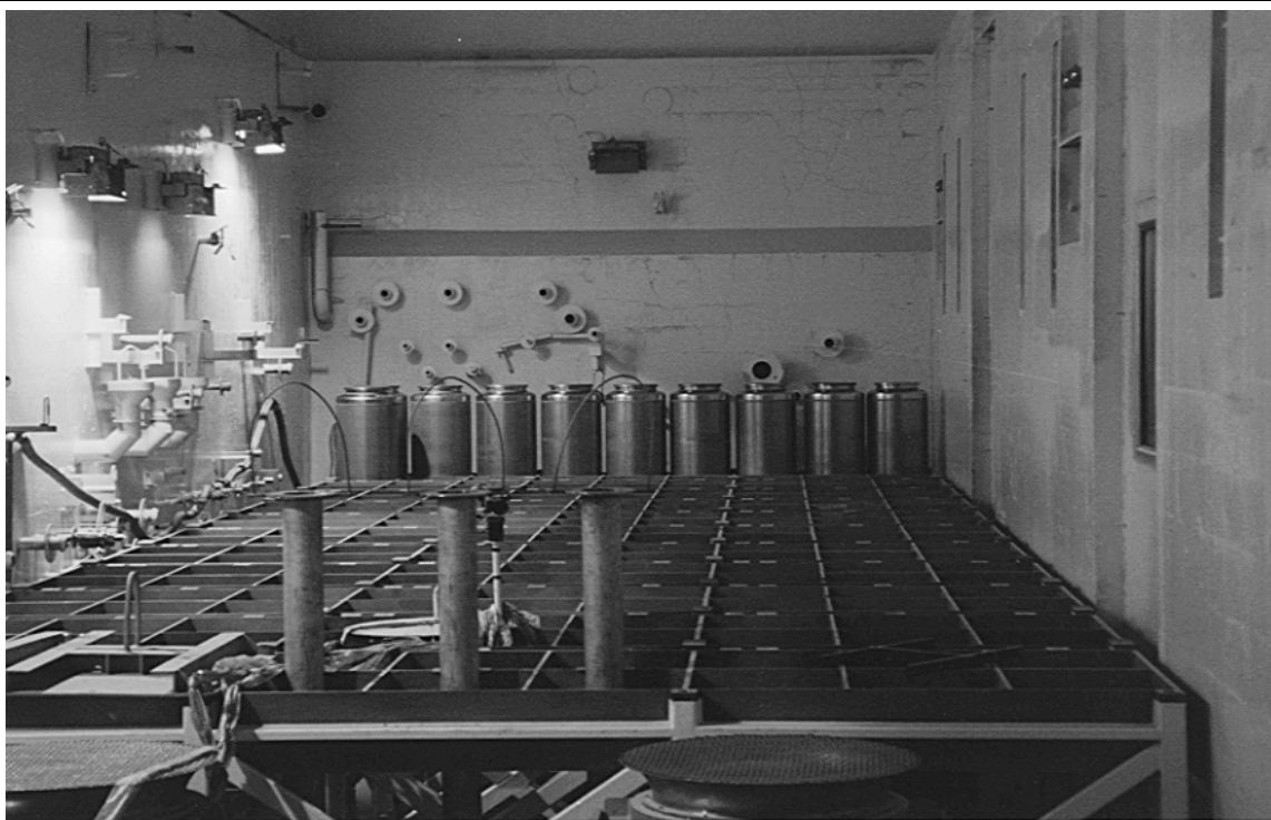
Fig. 31 - Stored vitrified canisters at West Valley
