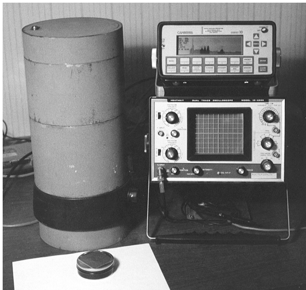
Fig. 32 - A radon canister counting setup
