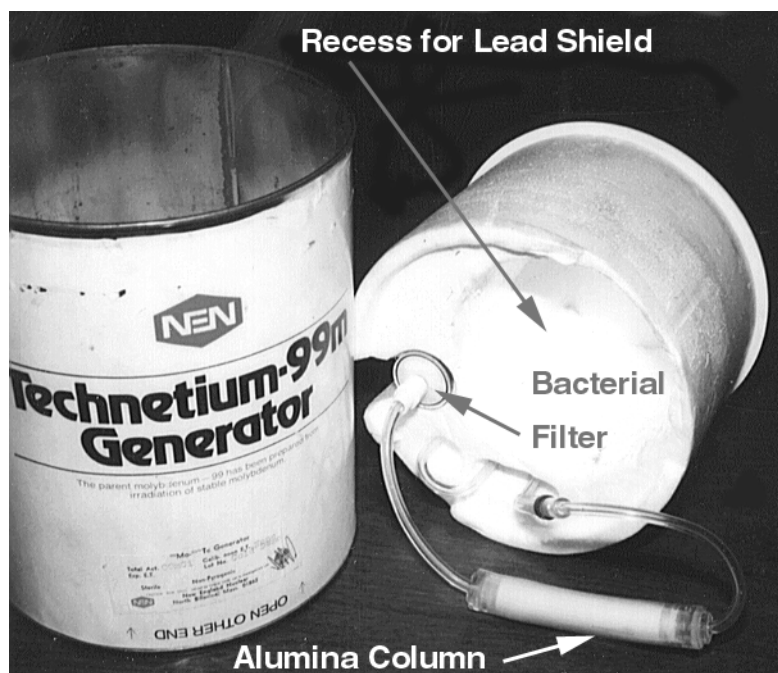
Fig. 45 - The insides of a "radioactive cow"
