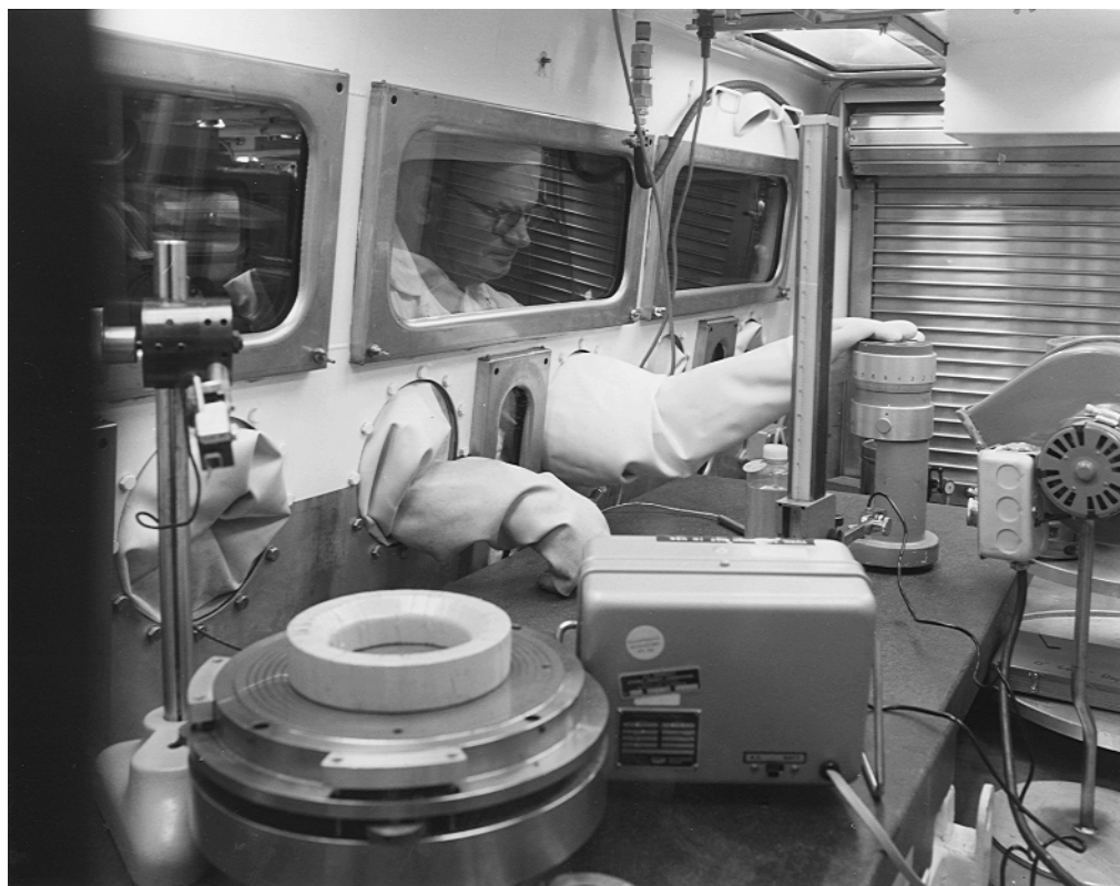
Fig. 89 - Rocky Flats glove box in use
