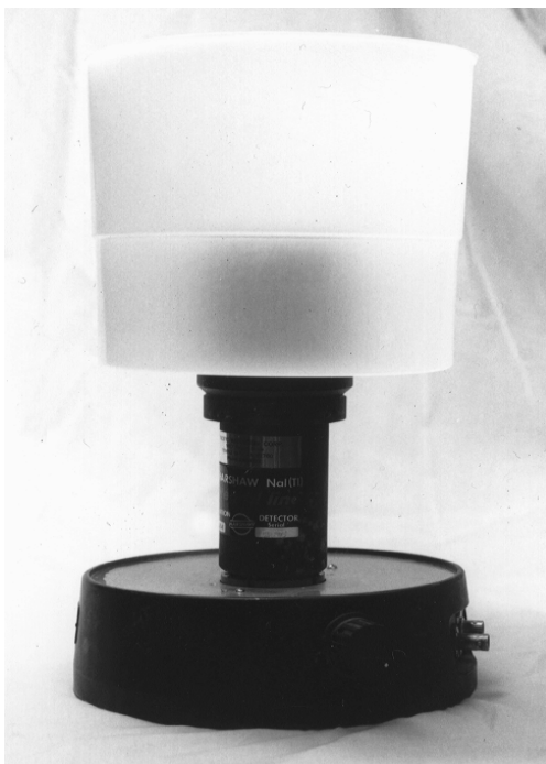
Fig. 37 - A Marinelli beaker and scintillation counter
