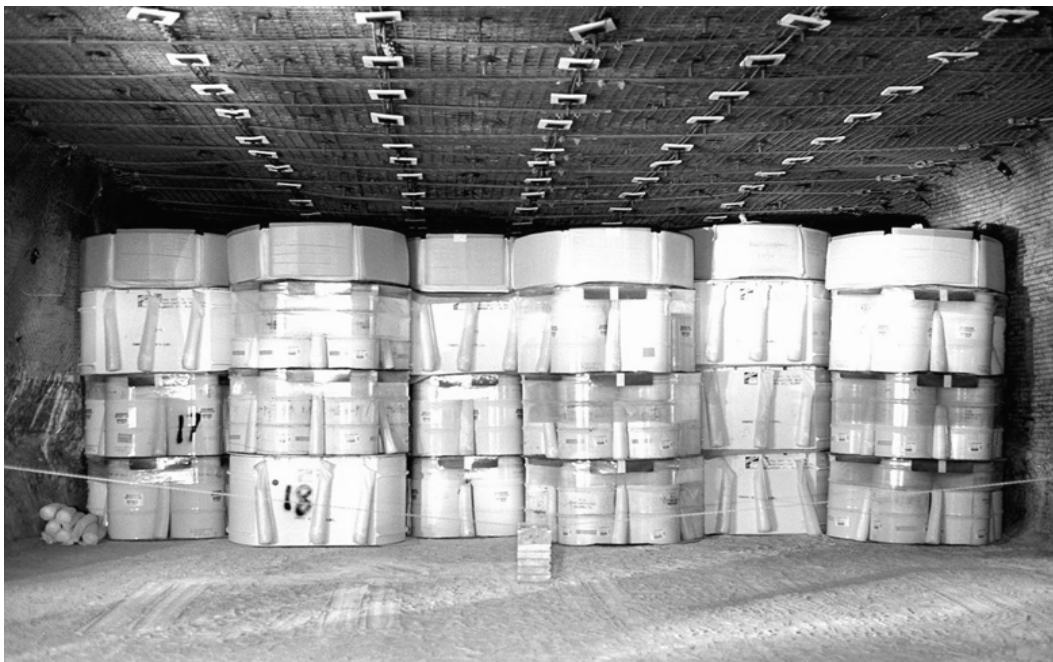
Fig. 44 - Final emplacement of transuranic waste in the WIPP salt deposit
