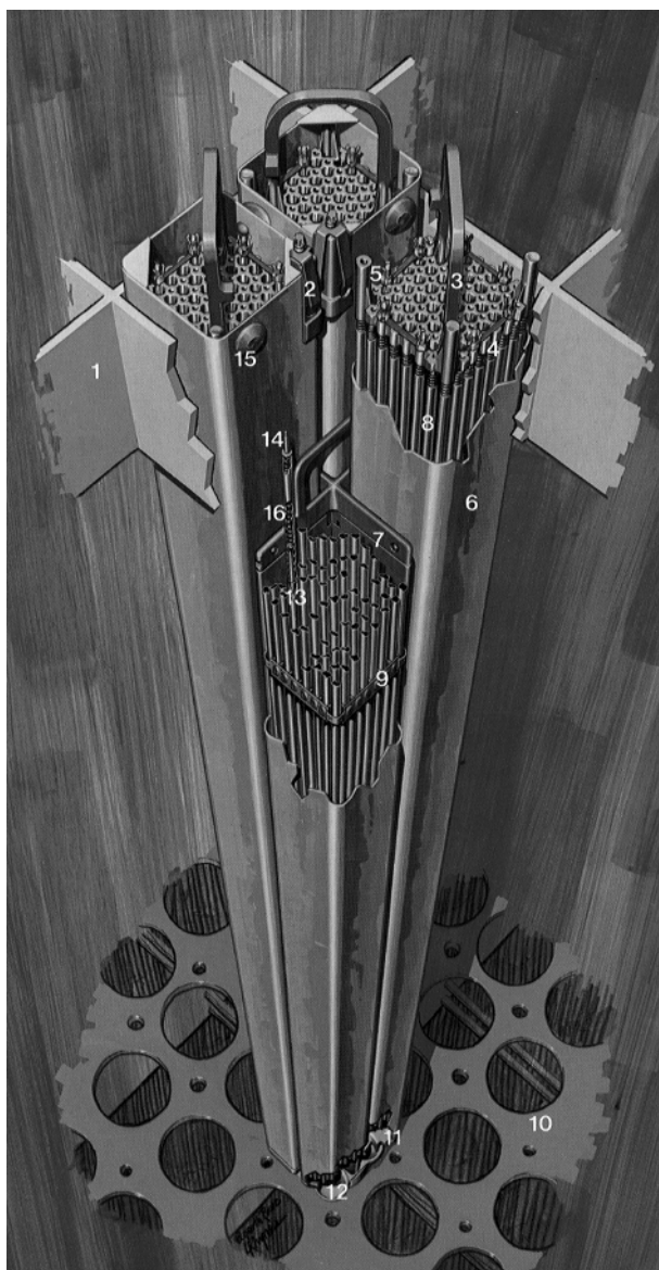
Fig. 14 - A BWR fuel assembly
